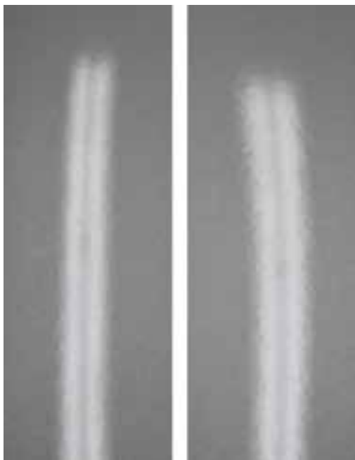
This image shows two panels. The sample on the left has an Ultragal® coating. Note the reflection of the fluorescent light. Waviness in the panel on the right (treated with Extragal®) is evidenced by the distorted reflection.
