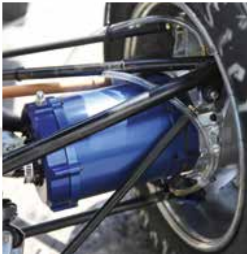
Each wheel is driven by an independent electric motor featuring iCARE® Save.
